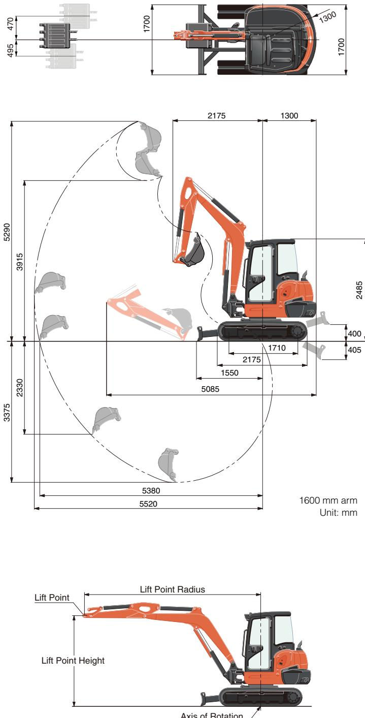
\* Working ranges are with Kubota standard bucket, without quick coupler.
